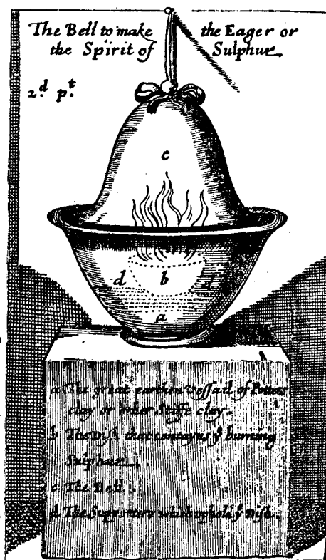
FIG. 3. THE BELL OR PER CAMPANAM METHOD OF MAKING SPIRIT OF SULPHUR. From Le Fevre, Compleat Body of Chymistry , 1664.
